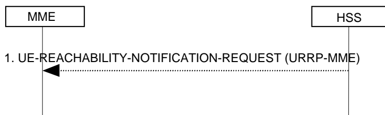
Figure 5.3.11.2-1: UE Reachability Notification Request Procedure
