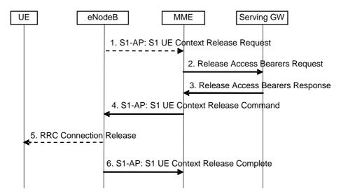
Figure 5.3.5-1: S1 Release Procedure
