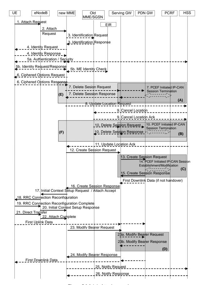
Figure 5.3.2.1-1: Attach procedure
