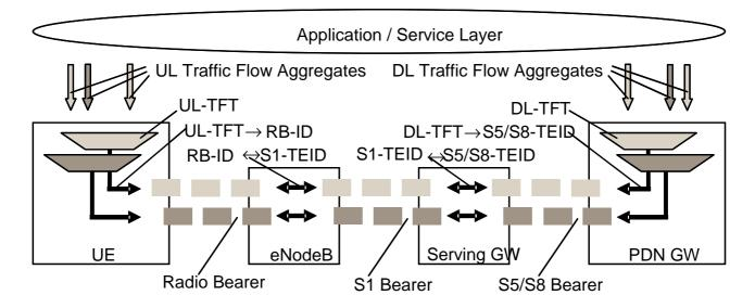
Figure 4.7.2.2-1: Two Unicast EPS bearers (GTP-based S5/S8)
