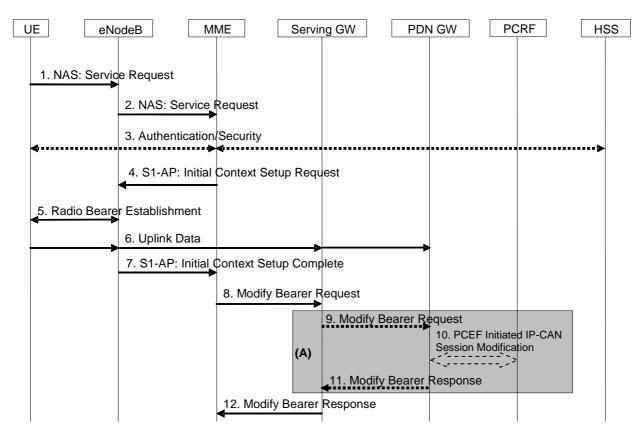
Figure 5.3.4.1-1: UE triggered Service Request procedure
