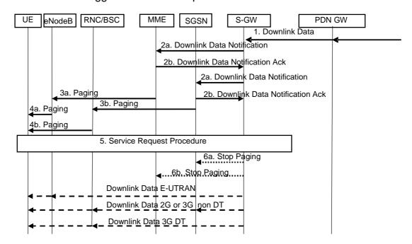
Figure 5.3.4.3-1: Network triggered Service Request procedure
