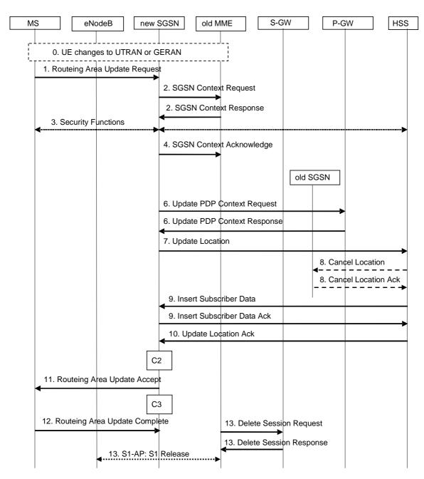
Figure D.3.5-1: Routing Area Update procedure
