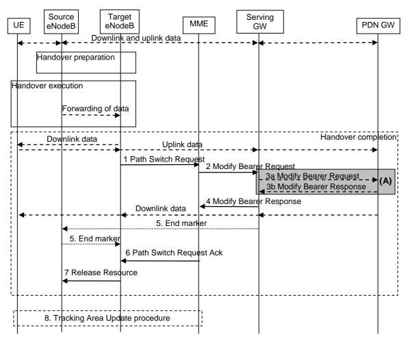
Figure 5.5.1.1.2-1: X2-based handover without Serving GW relocation
