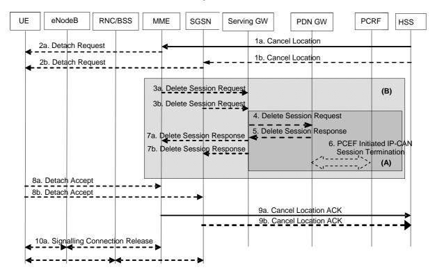
Figure 5.3.8.4-1: HSS-Initiated Detach Procedure
