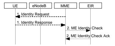
Figure 5.3.10.5-1: Identity Check Procedure
