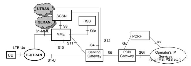
Figure 4.2.1-1: Non-roaming architecture for 3GPP accesses
