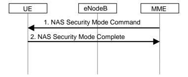
Figure 5.3.10.4.2-1: NAS Security Mode Command Procedure
