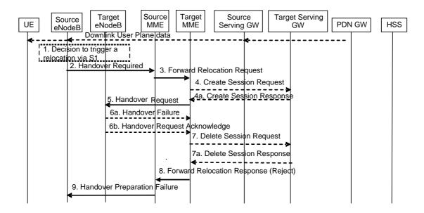
Figure 5.5.1.2.3-1: S1-based handover, Reject
