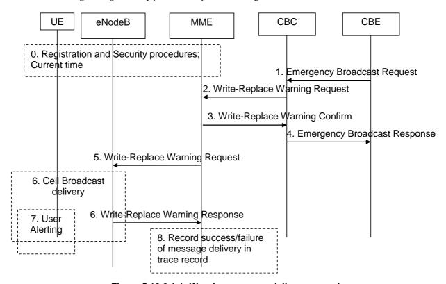
Figure 5.12.2.1-1: Warning message delivery procedure
