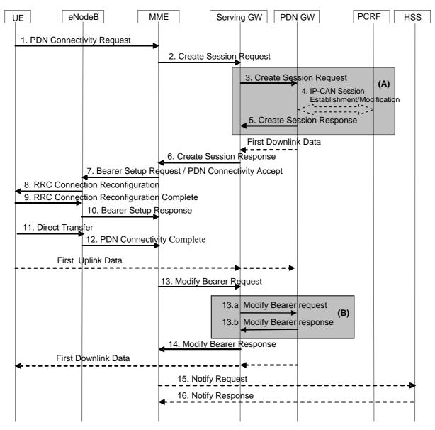
Figure 5.10.2-1: UE requested PDN connectivity
