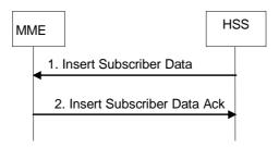
Figure 5.3.9.2-1: Insert Subscriber Data procedure
