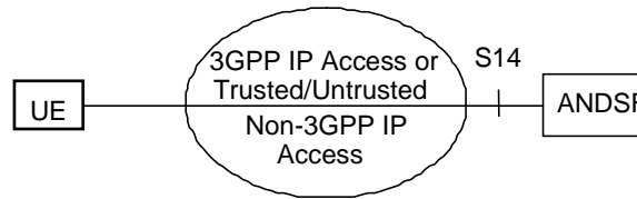
Figure 4.8.1.1-1: Architecture for Access Network Discovery Support Functions
