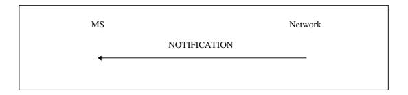
Figure 6.9a/3GPP TS 24.008: Notification procedure
