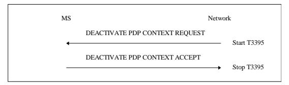
Figure 6.9/3GPP TS 24.008: Network initiated PDP context deactivation procedure
