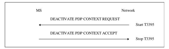
Figure 6.11/3GPP TS 24.008: MBMS context deactivation procedure
