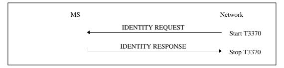
Figure 4.7.8/1 3GPP TS 24.008: Identification procedure
