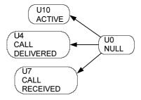
Figure 5.1a.2/3GPP TS 24.008: Overview call control protocol/MS side, extension for SRVCC from PS to CS
