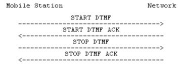
Figure 5.8/3GPP TS 24.008 Single DTMF transmission
