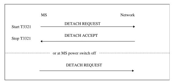
Figure 4.7.4/1 3GPP TS 24.008: MS initiated GPRS detach procedure
