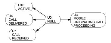
Figure 5.1a.2/3GPP TS 24.008: Overview call control protocol/MS side, extension for SRVCC from PS to CS
