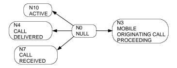
Figure 5.1b.2/3GPP TS 24.008: Overview call control protocol/Network side, extension for SRVCC from PS to CS
