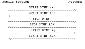
Figure 5.9/3GPP TS 24.008 Multiple DTMF transmission
