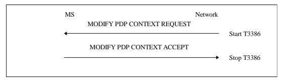
Figure 6.6/3GPP TS 24.008: Network initiated PDP context modification procedure
