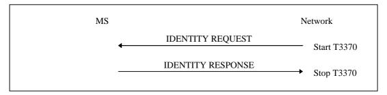
Figure 4.7.8/1 3GPP TS 24.008: Identification procedure
