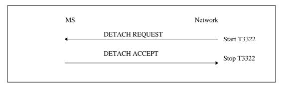
Figure 4.7.4/2 3GPP TS 24.008: Network initiated GPRS detach procedure
