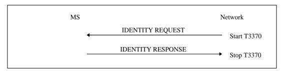
Figure 4.7.8/1 3GPP TS 24.008: Identification procedure
