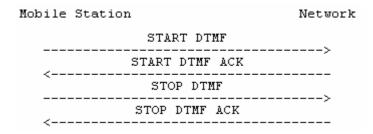
Figure 5.8/3GPP TS 24.008 Single DTMF transmission
