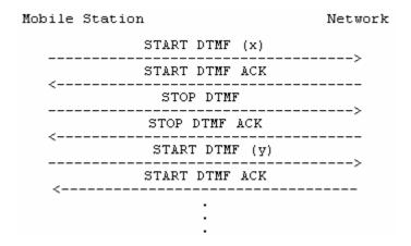
Figure 5.9/3GPP TS 24.008 Multiple DTMF transmission
