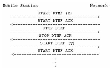
Figure 5.9/3GPP TS 24.008 Multiple DTMF transmission
