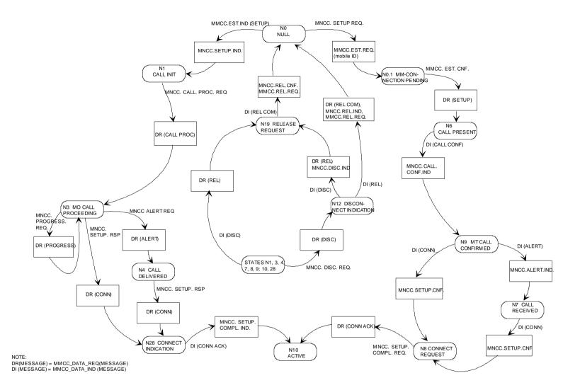
Figure 5.1b/3GPP TS 24.008 Overview call control protocol/Network side
