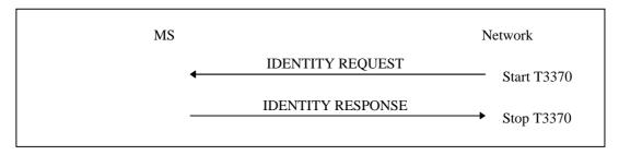
Figure 4.7.8/1 3GPP TS 24.008: Identification procedure
