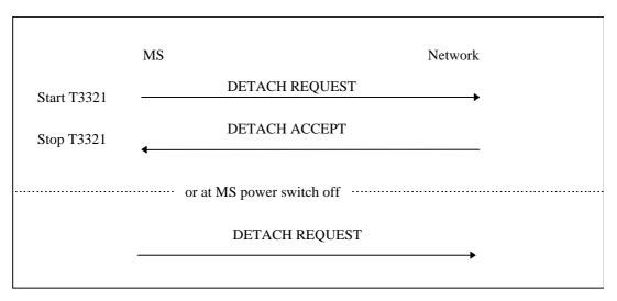
Figure 4.7.4/1 3GPP TS 24.008: MS initiated GPRS detach procedure
