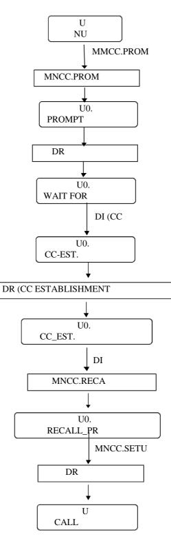
Figure 5.1a.1/3GPP TS 24.008: Overview call control protocol/MS side, extension:
