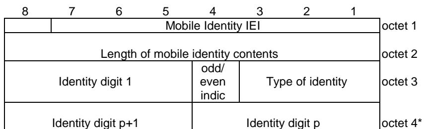
**Figure 10.5.4/3GPP TS 24.008 *Mobile Identity* information element**
