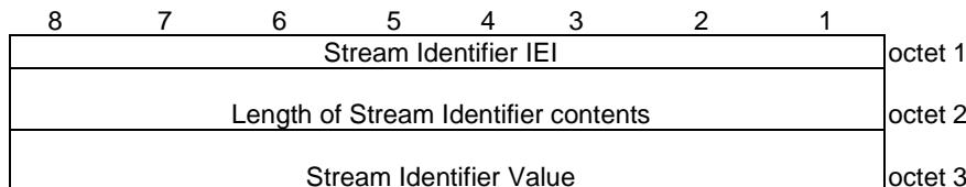
**Figure 10.5.117/3GPP TS 24.008: Stream Identifier information element**
