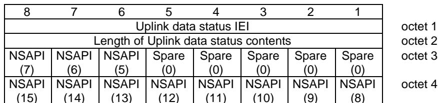
**Figure 10.5.149/3GPP TS 24.008 Uplink data status information element****Table 10.5.166/3GPP TS 24.008: Uplink data status information element**
