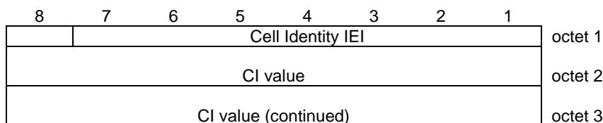
**Figure 10.5.1/3GPP TS 24.008 Cell Identity information element**
