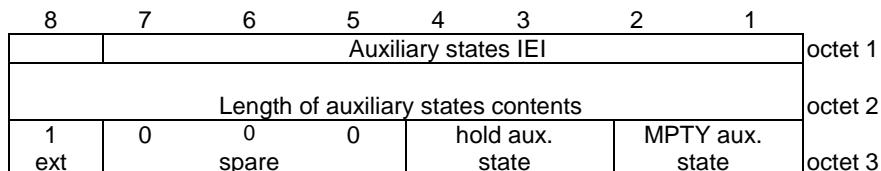
**Figure 10.5.87/3GPP TS 24.008 Auxiliary states information element****Table 10.5.100/3GPP TS 24.008: Auxiliary states information element**
