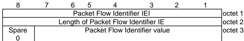
**Figure 10.5.143/3GPP TS 24.008: *Packet Flow Identifier* information element**
