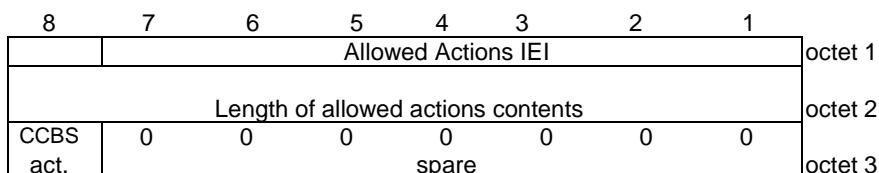
**Figure 10.5.116/3GPP TS 24.008 Allowed actions information element****Table 10.5.133/3GPP TS 24.008: Allowed actions information element**
