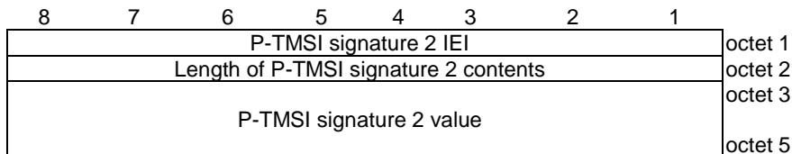
**Figure 10.5.124a/3GPP TS 24.008: *P-TMSI signature 2* information element****Table 10.5.141a/3GPP TS 24.008: *P-TMSI signature 2* information element**
