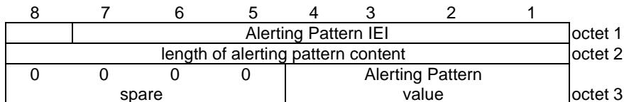
**Figure 10.5.115/3GPP TS 24.008 Alerting Pattern information element****Table 10.5.132/3GPP TS 24.008: Alerting Pattern information element**
