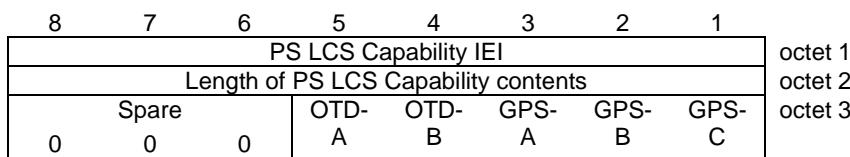
**Figure 10.5.135b/3GPP TS 24.008: PS LCS Capability information element**
