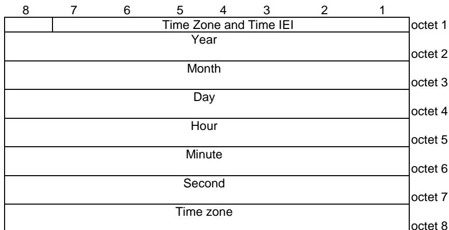
**Figure 10.5.84/3GPP TS 24.008 Time Zone and Time information element****Table 10.5.97/3GPP TS 24.008 Timezone and Time information element****Year (octet 2, bits 1-8)**
