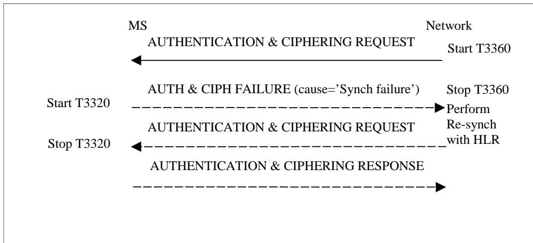
**Figure 4.7.7b/1 3GPP TS 24.008: Authentication failure cause "Synch failure"**
