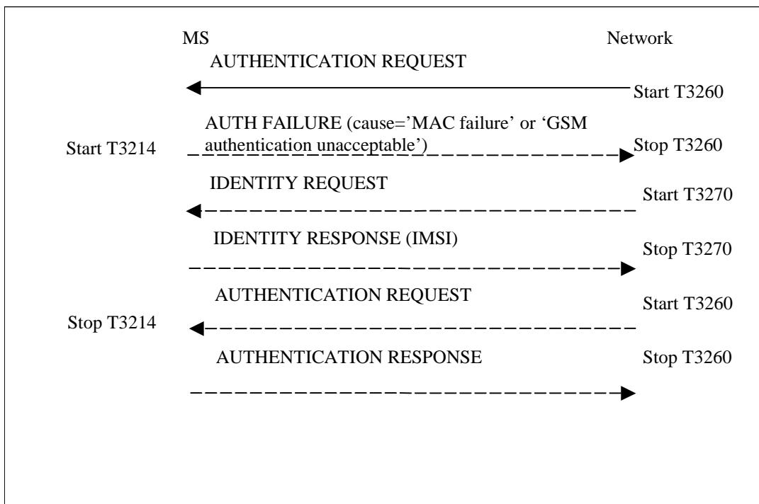
**Figure 4.2/3GPP TS 24.008: Authentication Failure Procedure
