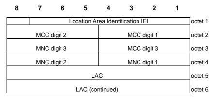
Figure 10.5.3/3GPP TS 24.008 Location Area Identification information element
