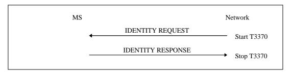
Figure 4.7.8/1 3GPP TS 24.008: Identification procedure
