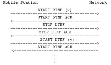
Figure 5.9/3GPP TS 24.008 Multiple DTMF transmission
