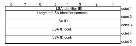
Figure 10.68c/3GPP TS 24.008 LSA Identifier information element
