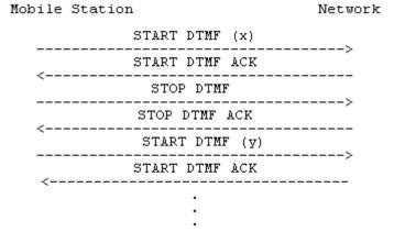
Figure 5.9/3GPP TS 24.008 Multiple DTMF transmission
