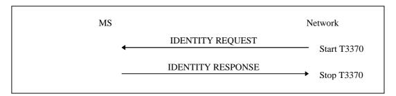
Figure 4.7.8/1 3GPP TS 24.008: Identification procedure
