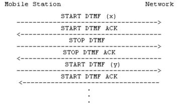
Figure 5.9/3GPP TS 24.008 Multiple DTMF transmission
