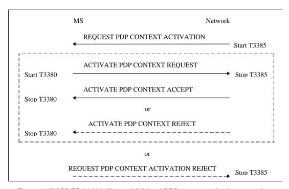
Figure 6.4/3GPP TS 24.008: Network initiated PDP context activation procedure
