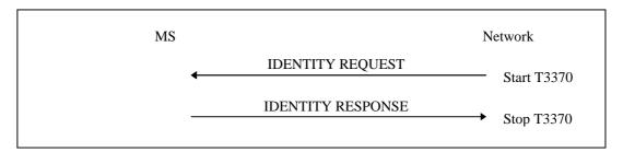
Figure 4.7.8/1 3GPP TS 24.008: Identification procedure
