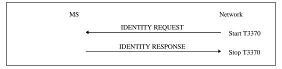
Figure 4.7.8/1 3GPP TS 24.008: Identification procedure
