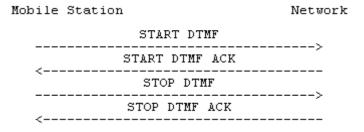
Figure 5.8/3GPP TS 24.008 Single DTMF transmission
