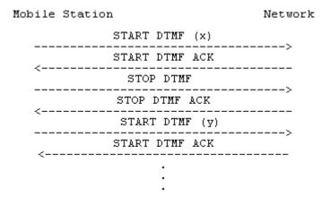
Figure 5.9/3GPP TS 24.008 Multiple DTMF transmission
