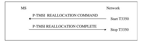
Figure 4.7.6/1 3GPP TS 24.008: P-TMSI reallocation procedure
