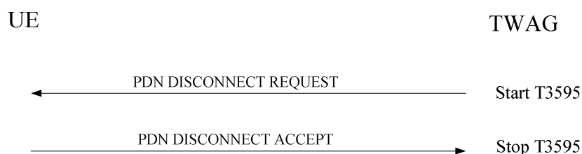
Figure 5.3.2.1: PDN disconnect procedure
