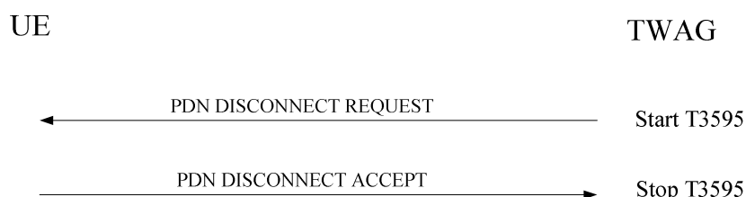
Figure 5.3.2.1: PDN disconnect procedure
