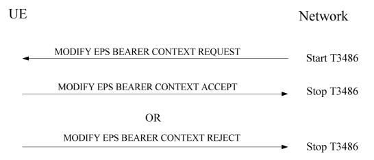
Figure 6.4.3.2.1: EPS bearer context modification procedure
