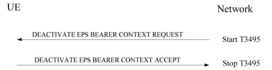
Figure 6.4.4.2.1: EPS bearer context deactivation procedure
