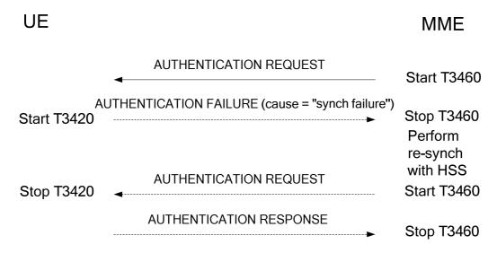
Figure 5.4.2.7.2: Authentication failure procedure (EMM cause #21 "synch failure")
