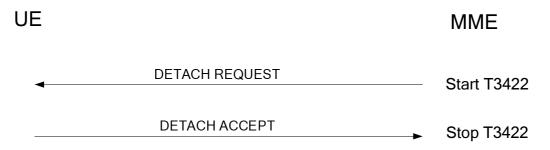
Figure 5.5.2.3.1: Network initiated detach procedure
