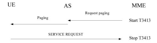
Figure 5.6.2.2.1.1: Paging procedure using S-TMSI
