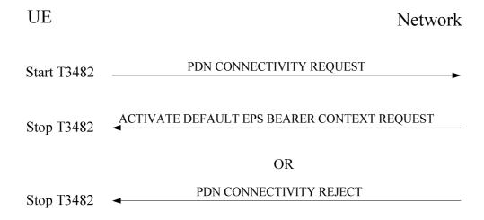
Figure 6.5.1.2.1: UE requested PDN connectivity procedure
