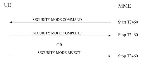
Figure 5.4.3.2.1: Security mode control procedure
