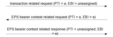
Figure 6.3.2.3: EPS bearer context related procedure triggered by a transaction related request
