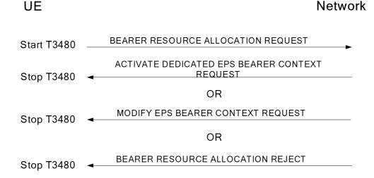
Figure 6.5.3.2.1: UE requested bearer resource allocation procedure
