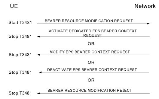
Figure 6.5.4.2.1: UE requested bearer resource modification procedure
