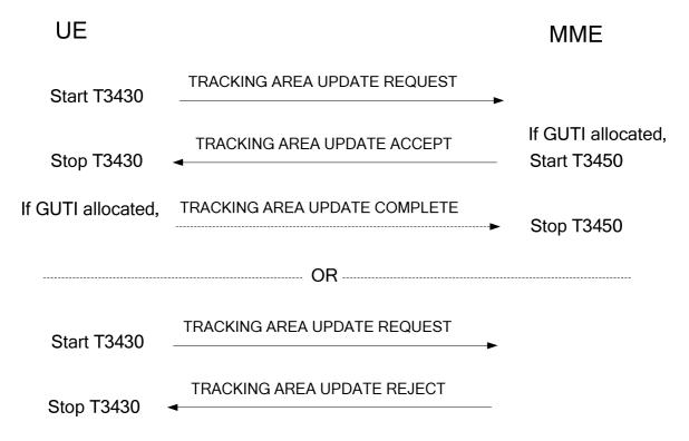
Figure 5.5.3.2.2.1: Tracking area updating procedure
