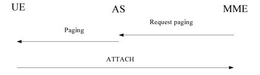
Figure 5.6.2.2.2.1: Paging procedure using IMSI
