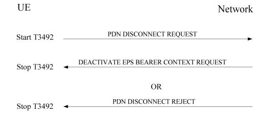
Figure 6.5.2.2.1: UE requested PDN disconnection procedure
