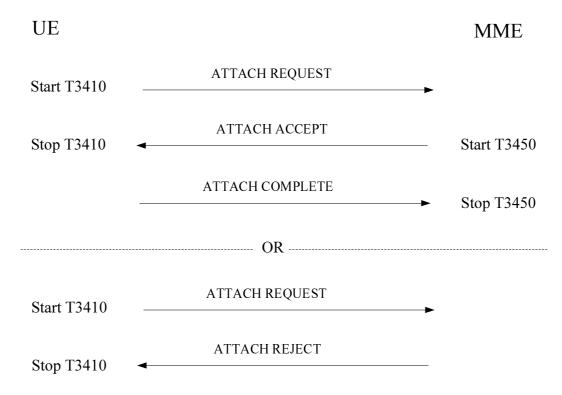
Figure 5.5.1.2.2.1: Attach procedure and combined attach procedure
