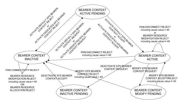
Figure 6.1.3.3.5.1: The ESM sublayer states for EPS bearer context handling in the network (overview)
