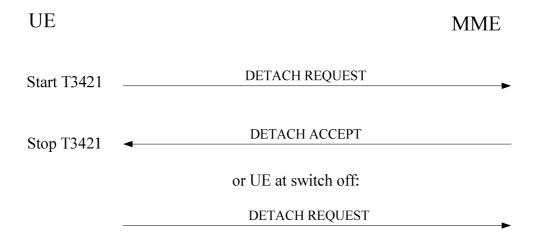
Figure 5.5.2.2.1.1: UE initiated detach procedure
