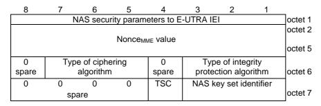
Figure 9.9.2.7.1: NAS security parameters to E-UTRA information element
