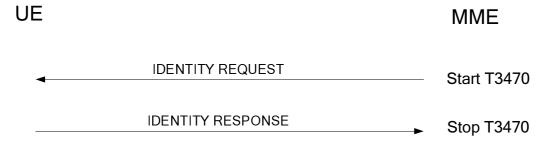
Figure 5.4.4.2.1: Identification procedure
