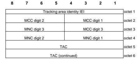
Figure 9.9.3.32.1: Tracking area identity information element
