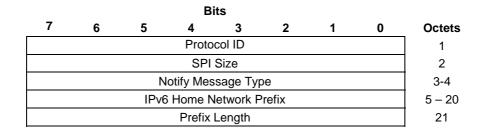
Figure B.1-1: PDN Identifier notify payload format
