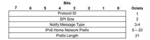
Figure B.1-1: PDN Identifier notify payload format
