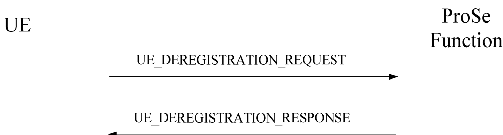
Figure 7.2.6.2.1.1: UE-initiated UE deregistration procedure
