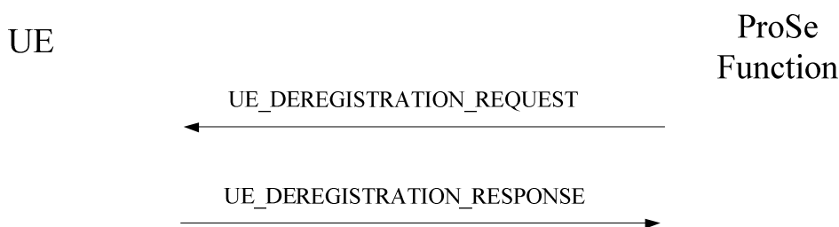
Figure 7.2.6.3.1.1: Network-initiated UE deregistration procedure
