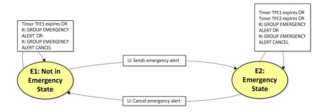
Figure 12.2.2.2-1: Emergency alert state machine
