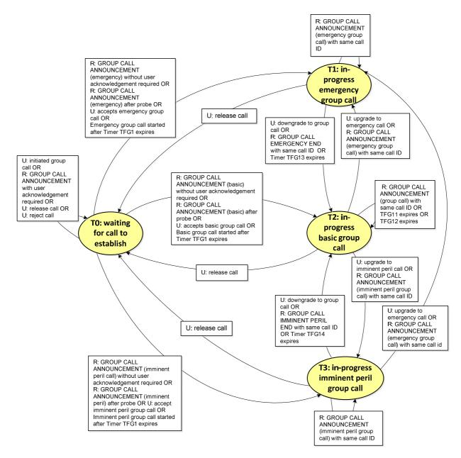
Figure 10.2.3.2-1: Call type control state machine
