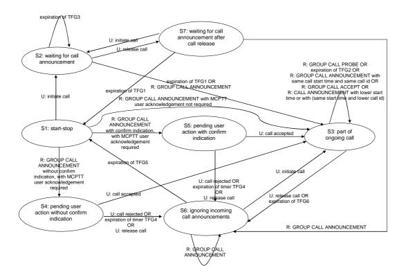
Figure 10.2.2.2-1: Basic call control state machine
