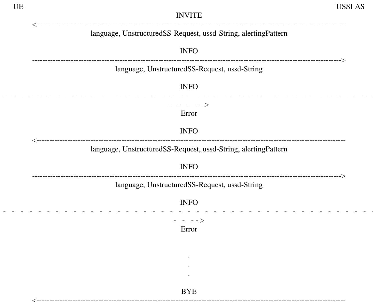
Figure 4.4: Multiple Network initiated USSD request
