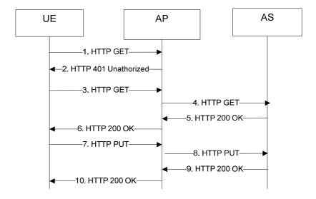
Figure A.7: Service configuration example
