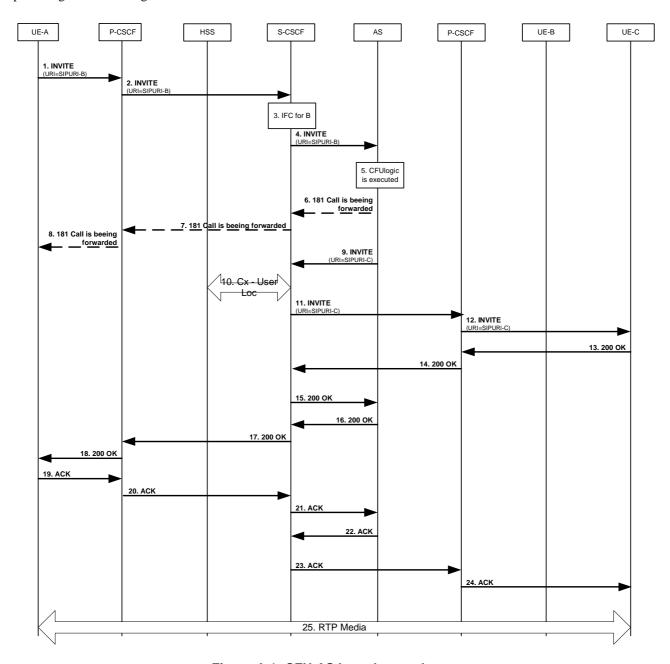
Figure A.1: CFU AS based normal case
