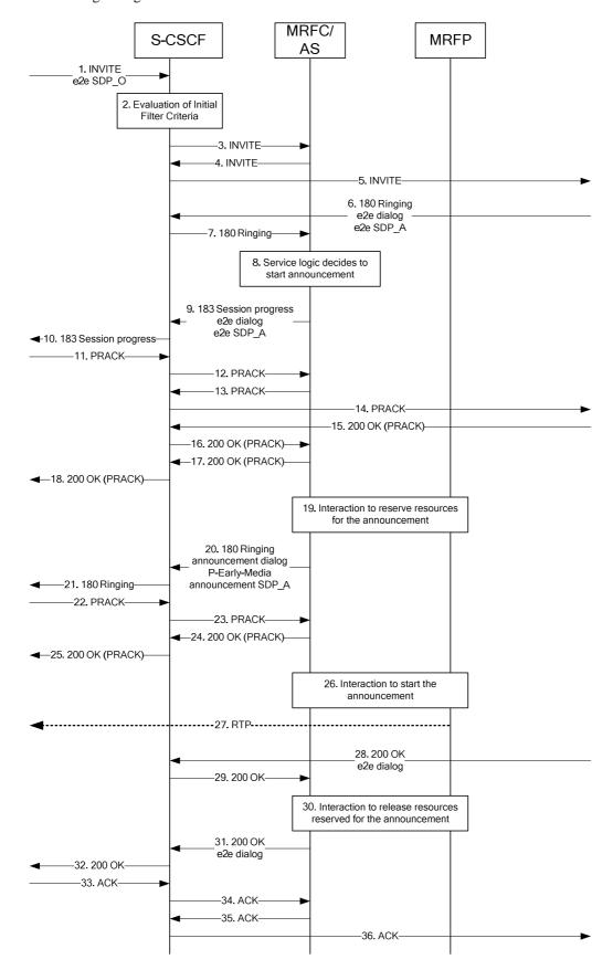
Figure A.5: Originating announcement during communication establishment considering terminating early media
