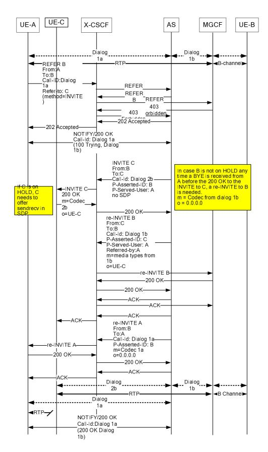
Figure E.5: Example flow for REFER interworking with REFER sent inside a dialog without usage of a media server
