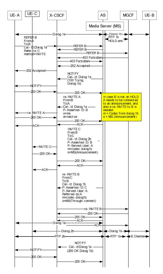
Figure E.1: Example flow for REFER interworking with REFER sent inside a dialog with usage of a media server
