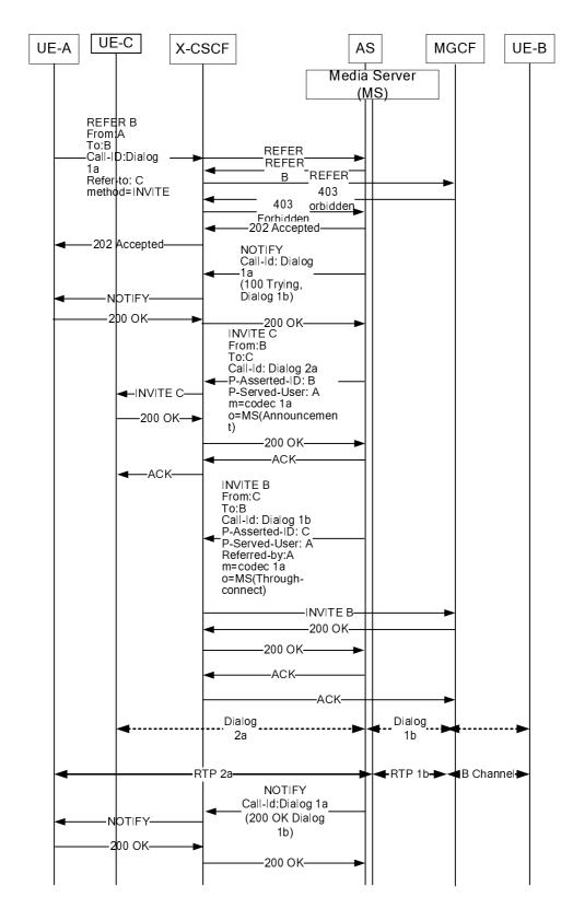
Figure E.2: Example flow for REFER interworking with REFER sent outside a dialog with usage of a media server
