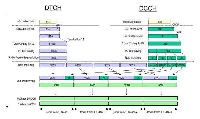
Figure A.4 (Informative): Channel coding of UL reference measurement channel (384 kbps)
