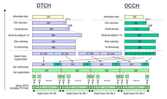
Figure A.5 (Informative): Channel coding of DL reference measurement channel (12.2 kbps)
