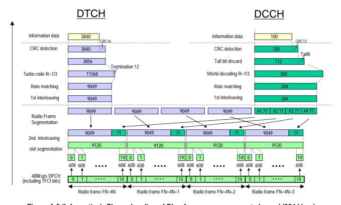
Figure A.8 (Informative): Channel coding of DL reference measurement channel (384 kbps)
