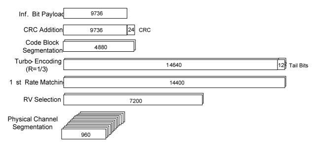
Figure A.25: Coding rate for Fixed Reference Channel H-Set 9 Secondary Transport Block
