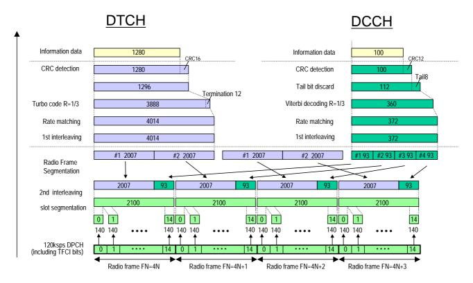
Figure A.6 (Informative): Channel coding of DL reference measurement channel (64 kbps)
