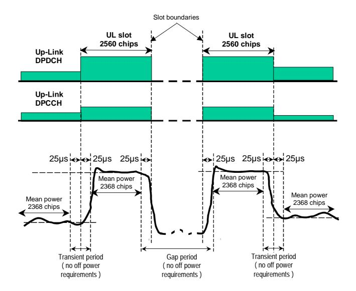
Figure 6.5: Transmit template during compressed mode
