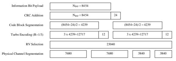
Figure A.4AB: E-DPDCH coding rate for DC-HSUPA reference measurement channel using 16QAM modulation
