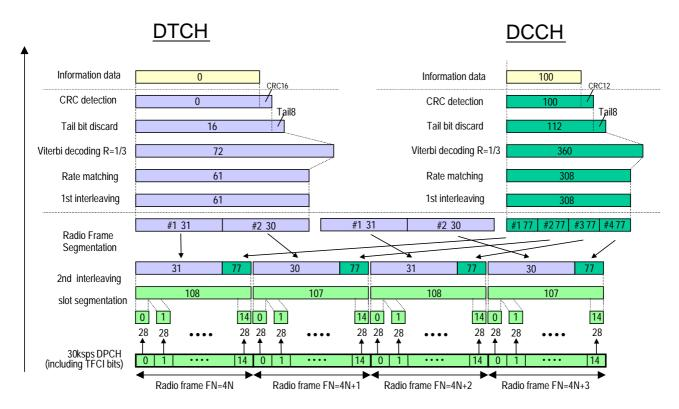
Figure A.4A (Informative): Channel coding of DL reference measurement channel (0 kbps)
