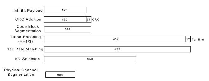
Figure A.28: Coding rate for Fixed reference Channel H-Set 12 (QPSK)
