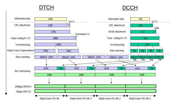
Figure A.2 (Informative): Channel coding of UL reference measurement channel (64 kbps)
