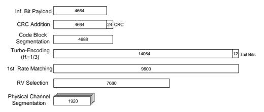
Figure A.15: Coding rate for Fixed Reference Channel H-Set 2 (16QAM)
