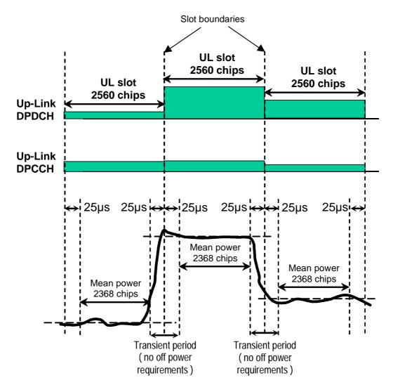
Figure 6.4: Transmit template during TFC change
