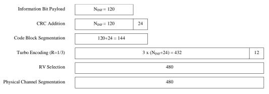
Figure A.4AA: E-DPDCH coding rate for DC-HSUPA reference measurement channel using BPSK modulation
