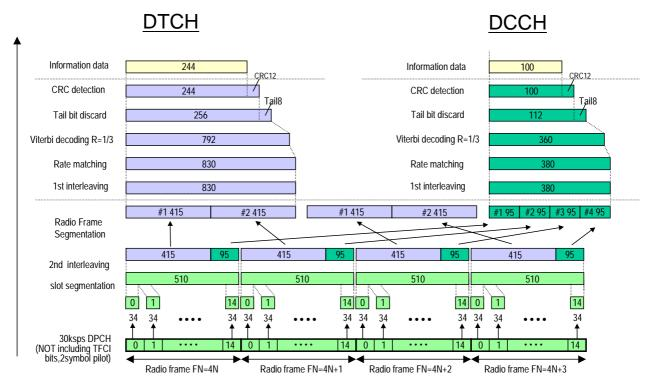
Figure A.9 (Informative): Channel coding of DL reference measurement channel for BTFD (Rate 1)
