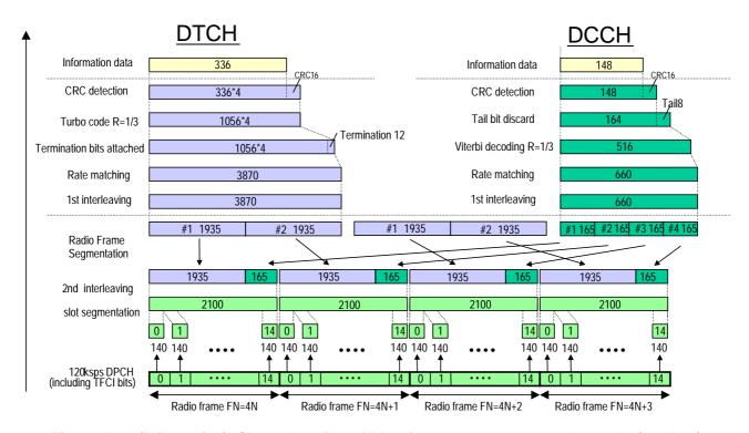
Figure A.8A (Informative): Channel coding of DL reference measurement channel 2 (64 kbps)
