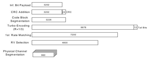
Figure A.18: Coding rate for Fixed Reference Channel H-Set 4
