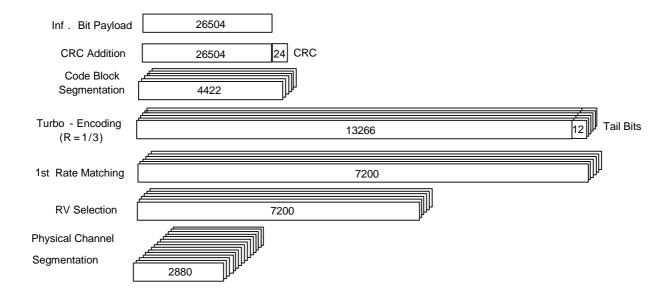
Figure A.26: Coding rate for Fixed Reference Channel H-Set 11 Primary Transport Block
