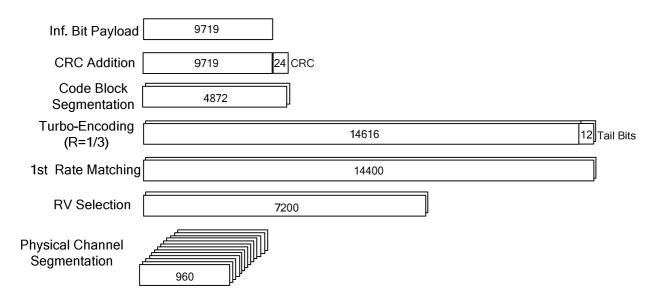
Figure A.25: Coding rate for Fixed Reference Channel H-Set 10 (QPSK)
