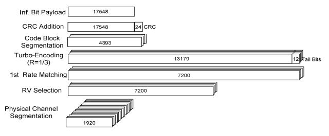
Figure A.24: Coding rate for Fixed Reference Channel H-Set 10 (16QAM)
