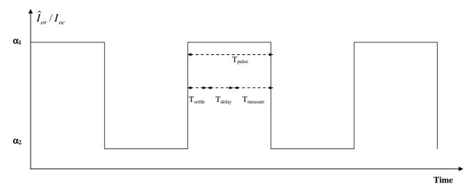
Figure 9.1 Test scenario for CQI reporting test under varying interference conditions.  $\hat{I}_{\sigma'}/I_{\sigma c}$  is varied between  $\alpha$ 1 and  $\alpha$ 2 according to a predetermined square wave pattern.
