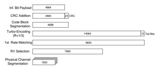
Figure A.13: Coding rate for Fixed reference Channel H-Set 1 (16 QAM)
