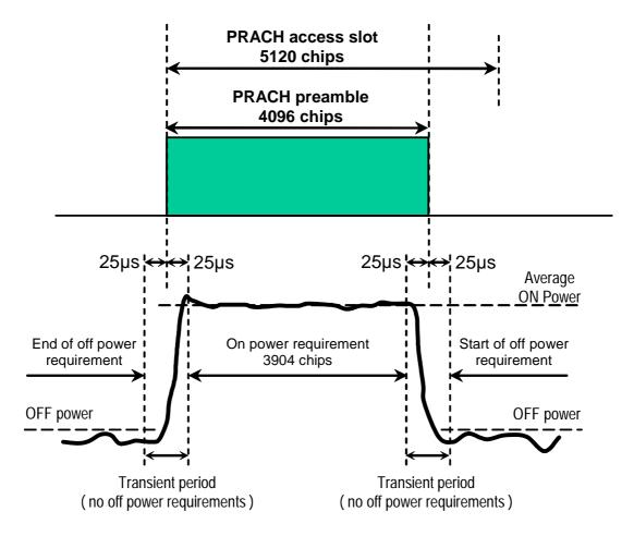
Figure 6.2: Transmit ON/OFF template for PRACH preambles
