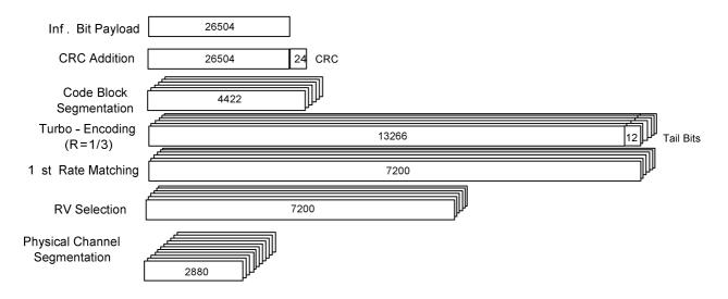
Figure A.23: Coding rate for Fixed reference Channel H-Set 8 (64 QAM)
