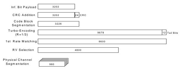
Figure A.19: Coding rate for Fixed Reference Channel H-Set 5
