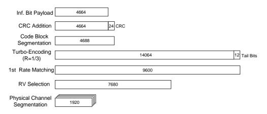
Figure A.17: Coding rate for Fixed reference Channel H-Set 3 (16QAM)
