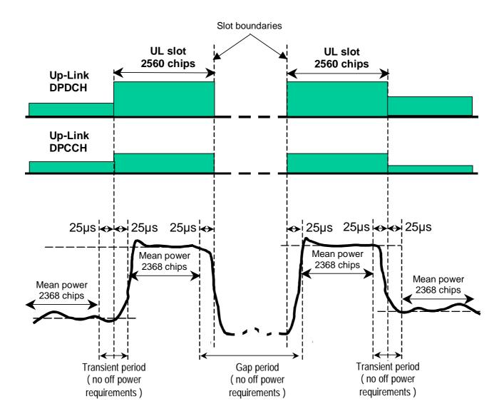
Figure 6.5: Transmit template during compressed mode
