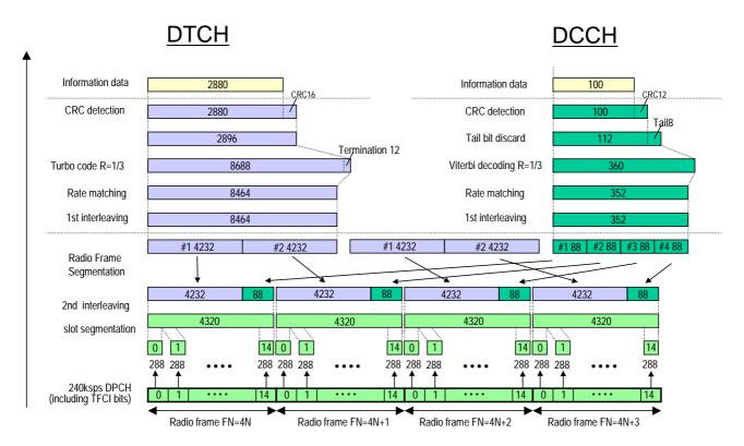
Figure A.7 (Informative): Channel coding of DL reference measurement channel (144 kbps)
