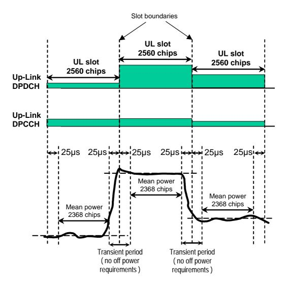
Figure 6.4: Transmit template during TFC change
