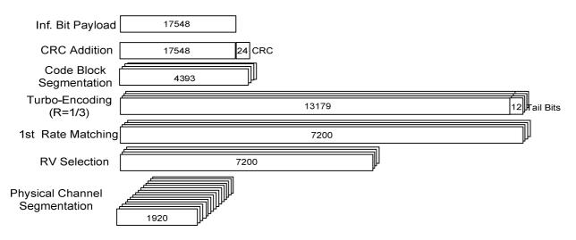
Figure A.24: Coding rate for Fixed Reference Channel H-Set 10 (16QAM)
