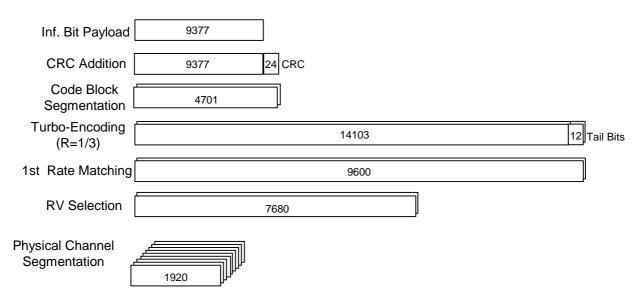
Figure A.21: Coding rate for Fixed reference Channel H-Set 6 (16 QAM)
