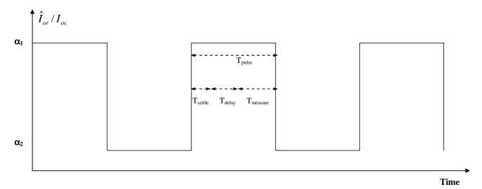
Figure 9.1 Test scenario for CQI reporting test under varying interference conditions.  $\hat{I}_{or}/I_{oc}$  is varied between  $\alpha$ 1 and  $\alpha$ 2 according to a predetermined square wave pattern.
