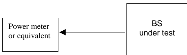
Figure B.1: Measuring system Set-up for maximum output power, total power dynamic range
