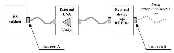
Figure 7.1: Receiver test ports
