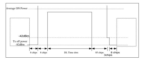
Figure 6.1A: Transmit ON/OFF template for 1,28 Mcps TDD option
