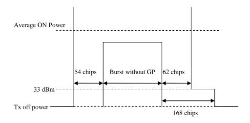
Figure 6.1B: Transmit ON/OFF template
