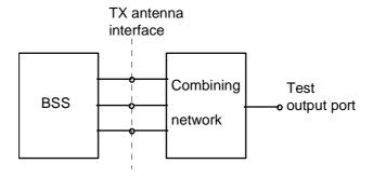
Figure 5.2: Transmitter test setup
