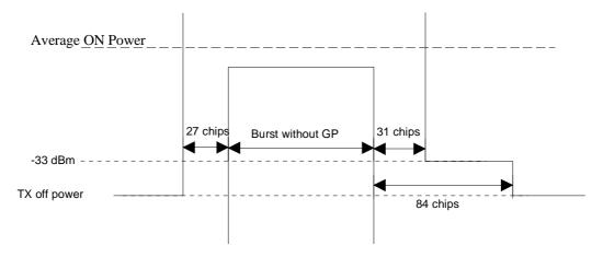
Figure 6.1: Transmit ON/OFF template
