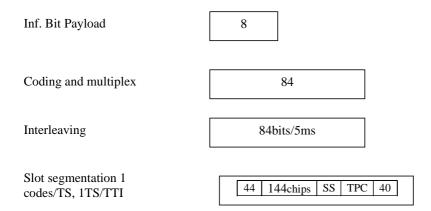
Figure A.19: Coding for HS-SICH type1 channel (1,28 Mcps TDD Option)
