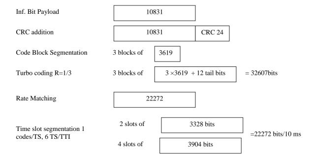
Figure A.11: Coding for E-DCH FRC2 (3,84 Mcps TDD Option)
