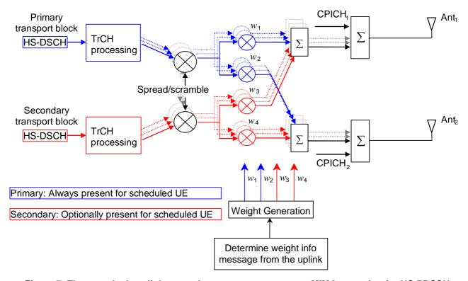
Figure 7: The generic downlink transmitter structure to support MIMO operation for HS-PDSCH transmission.
