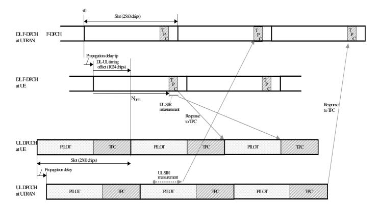
Figure B.4: Transmitter power control timing for F-DPCH with a TPC offset N<sub>OFF1</sub> larger than 14 with uplink DPCCH slot format #4
