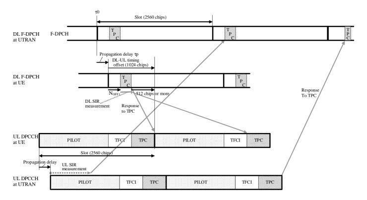
Figure B.2a: Transmitter power control timing for F-DPCH with TPC offsets  $N_{OFF1}$  of 0 or 2 when the F-DPCH TPC offset  $N_{OFF1}$  of at least one other radio link in the RLS is > 2
