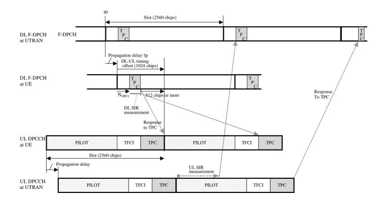
Figure B.2: Transmitter power control timing for F-DPCH with TPC offsets N<sub>OFF1</sub> of 0 or 2 when F-DPCH TPC offset N<sub>OFF1</sub> of all the radio links in the RLS is 0 or 2
