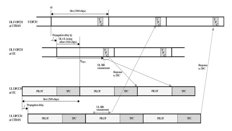
Figure B.4: Transmitter power control timing for F-DPCH with a TPC offset N<sub>OFF1</sub> larger than 14 with uplink DPCCH slot format #4
