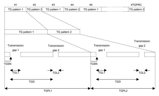
Figure 1: Illustration of compressed mode pattern parameters
