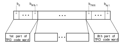
Figure 9A: Mapping of TFCI code word bits to TFCI position in 1.28 Mcps TDD option for downlink MBSFN, where  $N = N_{TFCI \text{ code word}}$ .
