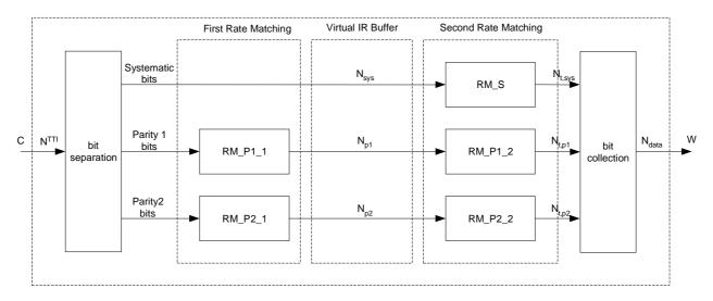
Figure 16: HS-DSCH hybrid ARQ functionality
