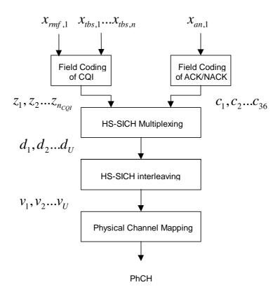
Figure 20: Coding and multiplexing for HS-SICH
