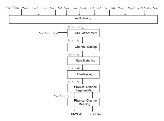
Figure 19E: Coding and Multiplexing for HS-SCCH type 6
