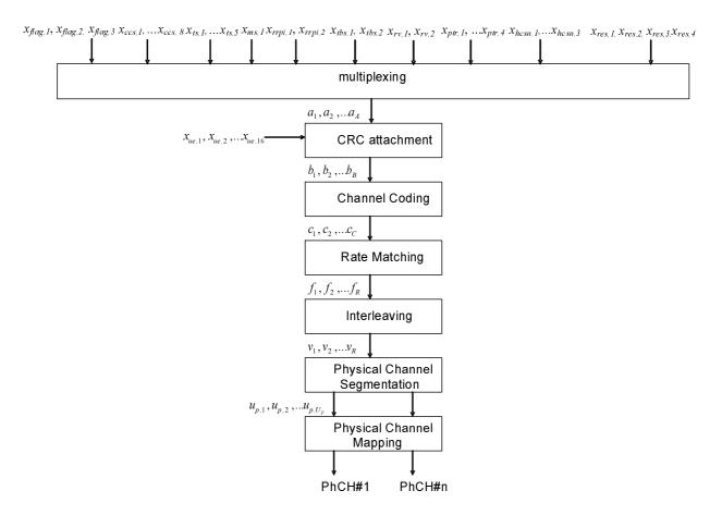
Figure 19F: Coding and Multiplexing for HS-SCCH type 7
