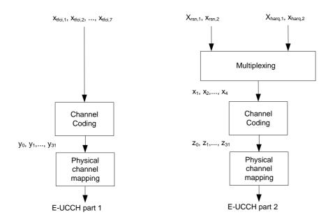
Figure 24: Coding chain for E-UCCH parts 1 and 2
