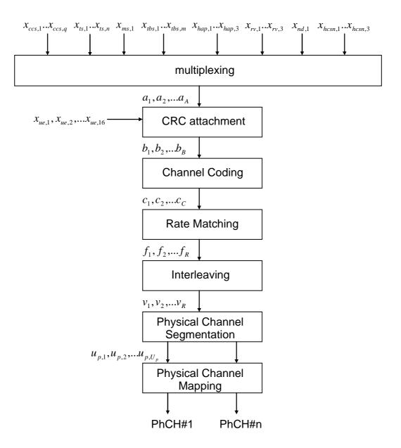
Figure 19 Coding and Multiplexing for HS-SCCH
