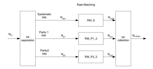
Figure 23: E-DCH hybrid ARQ functionality
