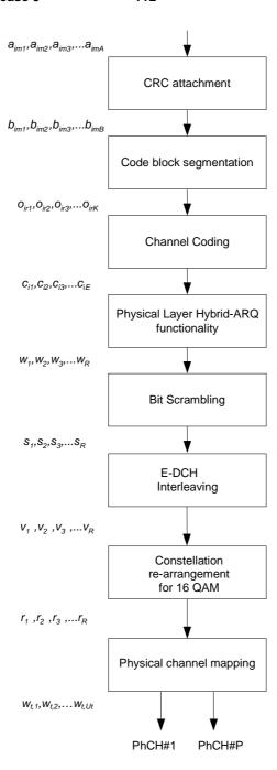
Figure 22. Coding chain for E-DCH
