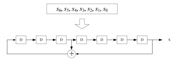
Figure 27: Structure of PN register
