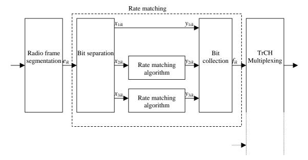
Figure 4: Puncturing of turbo encoded TrCHs
