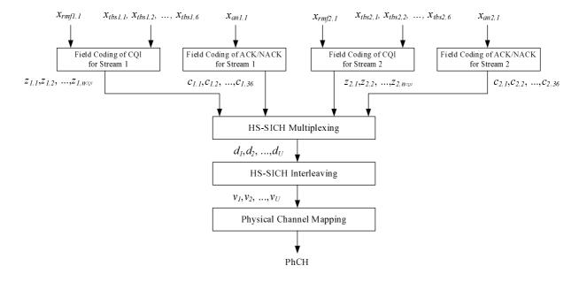
Figure 20A: Coding and multiplexing for HS-SICH type 2
