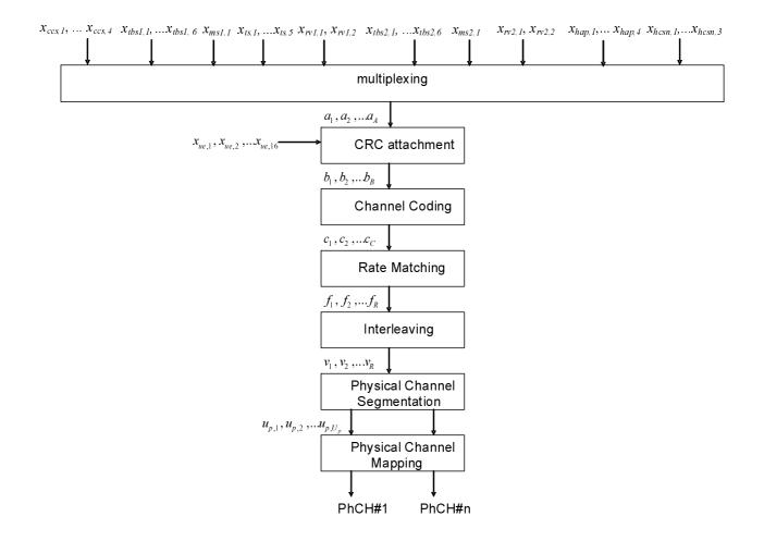
Figure 19H: Coding and Multiplexing for HS-SCCH type 9
