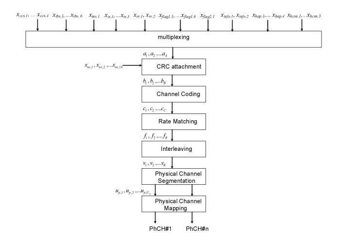
Figure 19G: Coding and Multiplexing for HS-SCCH type 8
