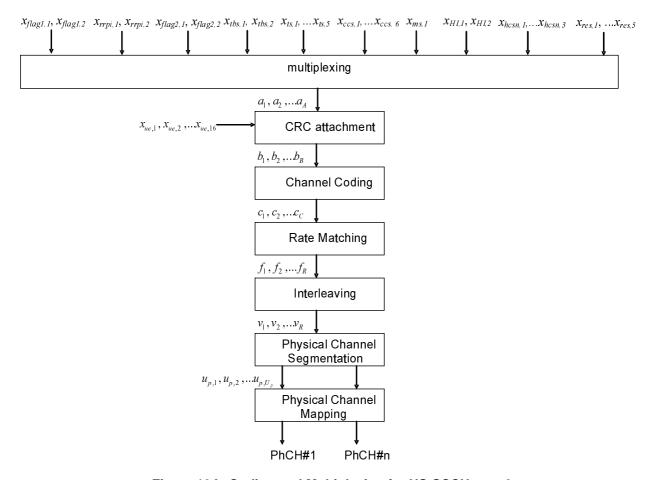
Figure 19A: Coding and Multiplexing for HS-SCCH type 2
