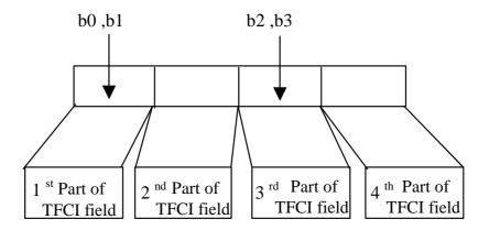
Figure 10: Mapping of TFCI code word bits to TFCI position in 1.28 Mcps TDD option, when N<sub>TFCI code word</sub>=4
