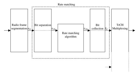
Figure 5: Rate matching for uncoded TrCHs, convolutionally encoded TrCHs, and for turbo encoded TrCHs with repetition
