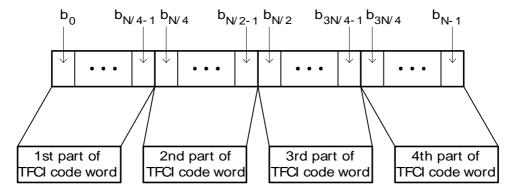
Figure 13: Mapping of TFCI code word bits to timeslot in 1.28 Mcps TDD option, where  $N = N_{TFCI \text{ code word}}$ .
