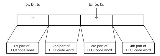
Figure 14: Mapping of TFCI code word bits to timeslot in 1.28 Mcps TDD option when N<sub>TFCI code word</sub> = 6
