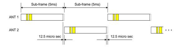
Figure 7: Example for the antenna swithing pattern for TSTD transmission of DPCH/PDSCH and P-CCPCH: all physical channels are transmitted with TSTD and are using the same antenna in the sub-frame.
