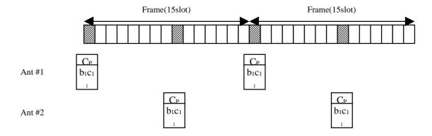
Figure 3: Antenna Switching Pattern (Case 2)
