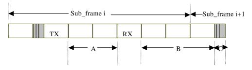
Figure A.2: Possible idle periods in a subframe with two occupied timeslots
