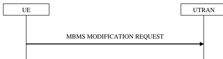
Figure 8.7.6-1: MBMS modification request, normal
