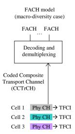
Figure 3: Model of the UE's physical layer - downlink FDD mode
