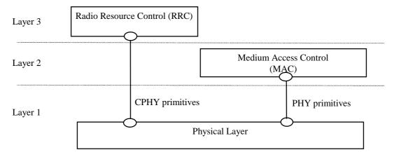
Figure 1: Interfaces with the Physical Layer
