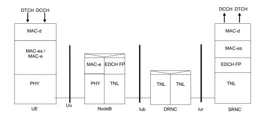
Figure 6.1-1: Protocol Architecture of E-DCH (MAC-e/es)
