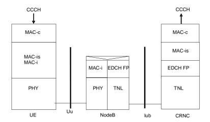
Figure 6.1-4: Protocol Architecture of E-DCH (MAC-i/is) for CCCH transmission
