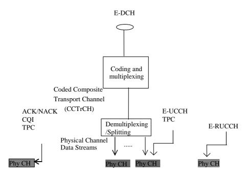
Figure 6.3.1.2-1: Model of the UE's Uplink physical layer
