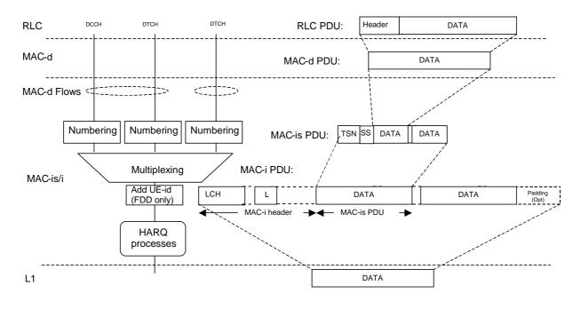
Figure 7.2.1-4: Simplified architecture showing MAC inter-working in UE when MAC-i/is is configured for DTCH and DCCH transmission. The left part shows the functional split while the right part shows PDU construction.
