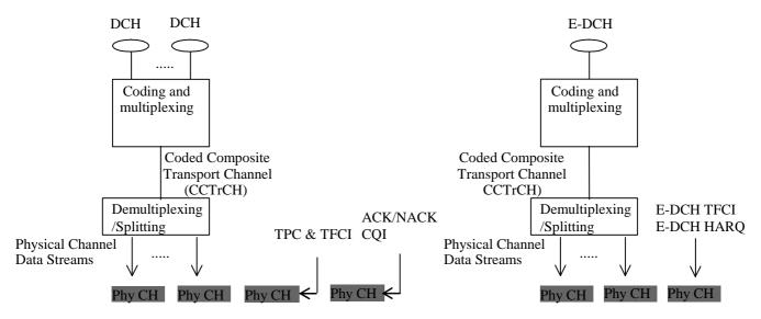
Figure 6.3.1.1-1: Model of the UE's Uplink physical layer
