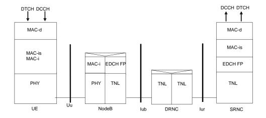
Figure 6.1-2: Protocol Architecture of E-DCH (MAC-i/is) for CELL\_DCH
