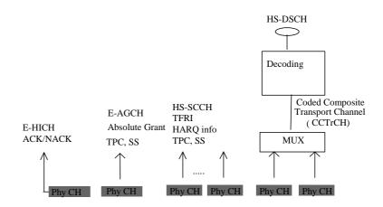
Figure 6.3.2.3-1: Model of the UE's Downlink physical layer (E-DCH model with HS-DSCH).
