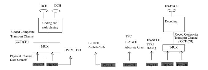
Figure 6.3.2.3-2: Model of the UE's Downlink physical layer (E-DCH with DCH and HS-DSCH).
