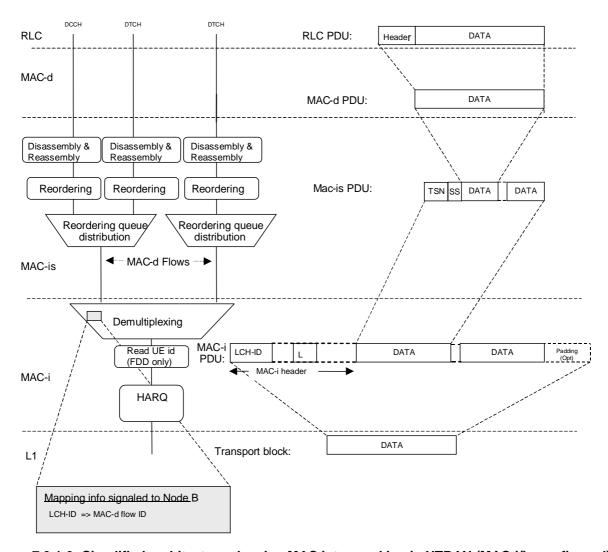
Figure 7.3.1-3: Simplified architecture showing MAC inter-working in UTRAN (MAC-i/is configured).
