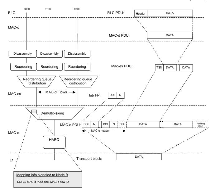
Figure 7.3.1-2: Simplified architecture showing MAC inter-working in UTRAN (MAC-e/es configured).
