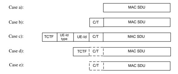
Figure 9.2.1.1.1: MAC PDU formats for DTCH and DCCH
