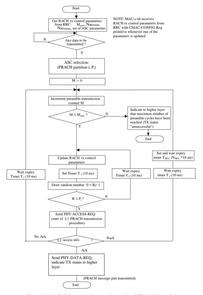
Figure 11.2.2.1: RACH transmission control procedure (UE side, informative)
