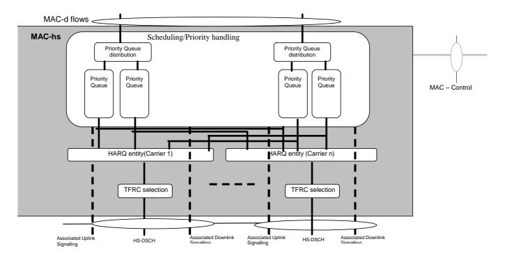
Figure 4.2.4.3.2: UTRAN side MAC architecture/MAC-hs details (1.28Mcps TDD multi-frequency HS-DSCH operation mode only)
