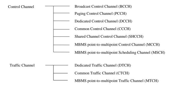
Figure 4.3.2.1: Logical channel structure
