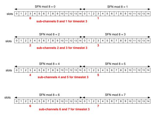
Figure 11.2.3.1 Eight sub-channels for timeslot 3
