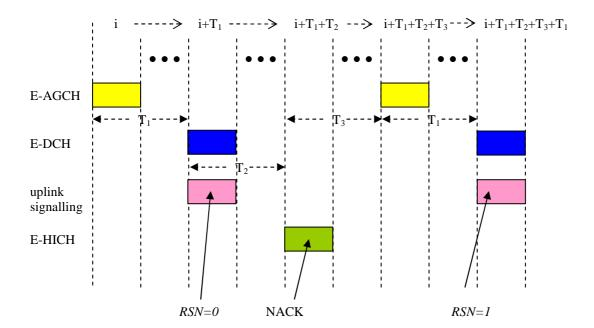
Figure 11.9.1.1: TDD E-DCH HARQ Operation
