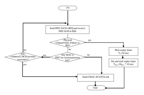
Figure 11.2.2A-2: Enhanced Uplink in CELL\_FACH state and Idle mode transmission control procedure (UE side, informative), Part II for CCCH transmission
