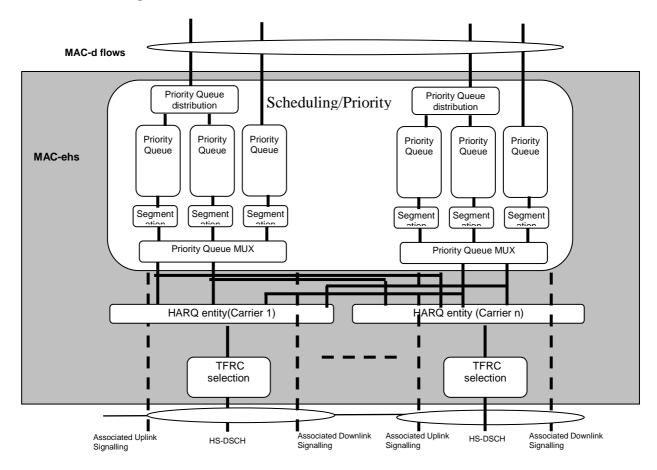
Figure 4.2.4.6-2: UTRAN side MAC architecture/MAC-ehs details (1.28Mcps TDD multi-frequency HS-DSCH operation mode only)
