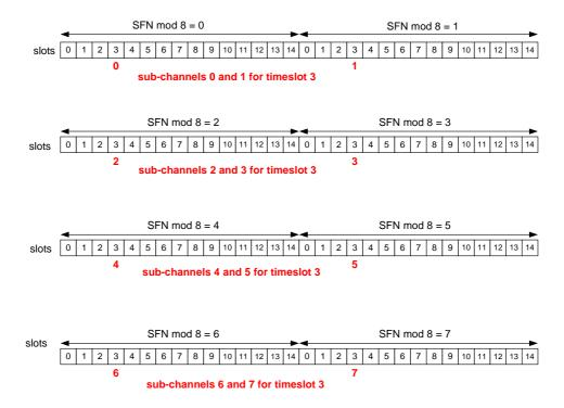
Figure 11.2.3.1 Eight sub-channels for timeslot 3
