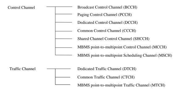
Figure 4.3.2.1: Logical channel structure
