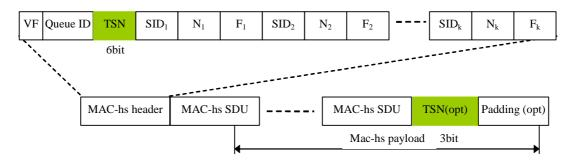
Figure 9.1.4.3: MAC-hs PDU (1.28Mcps TDD multi-frequency HS-DSCH operation mode only)
