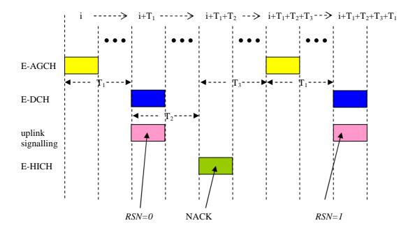
Figure 11.9.1.1: TDD E-DCH HARQ Operation
