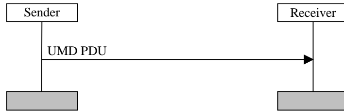
Figure 11.2: Unacknowledged mode data transfer procedure
