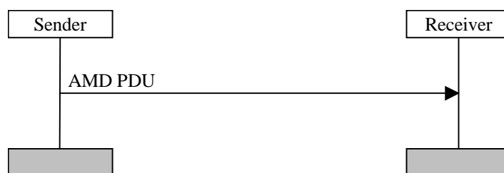
Figure 11.3: Acknowledged mode data transfer procedure
