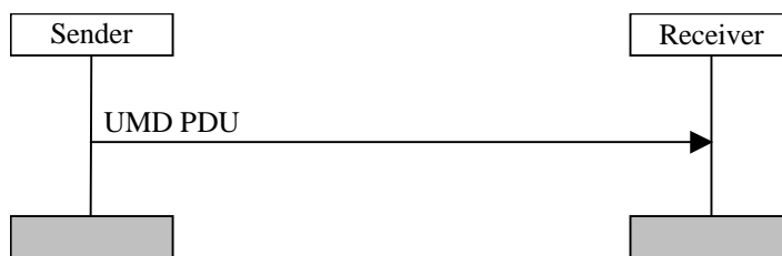
Figure 11.2: Unacknowledged mode data transfer procedure
