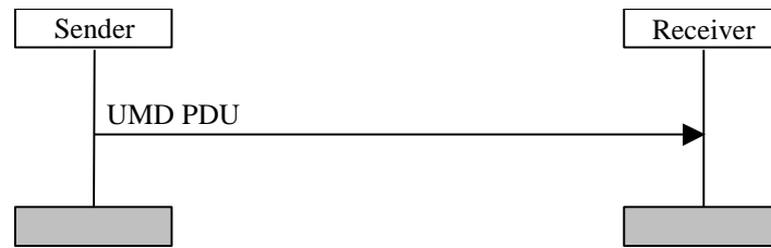
Figure 11.2: Unacknowledged mode data transfer procedure
