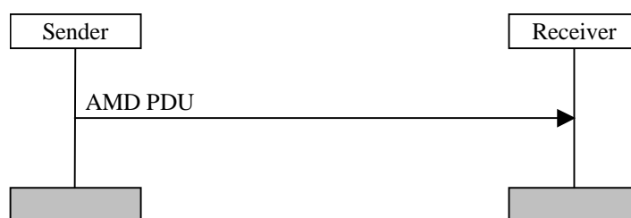
Figure 11.3: Acknowledged mode data transfer procedure
