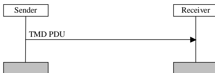
Figure 11.1: Transparent mode data transfer procedure
