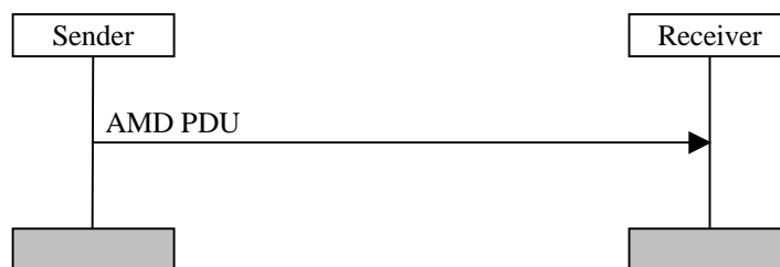
Figure 11.3: Acknowledged mode data transfer procedure
