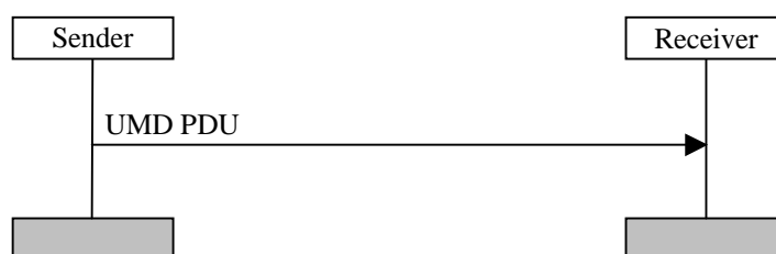
Figure 11.2: Unacknowledged mode data transfer procedure
