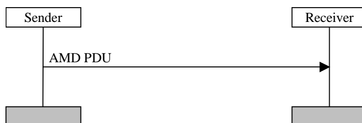
Figure 11.3: Acknowledged mode data transfer procedure
