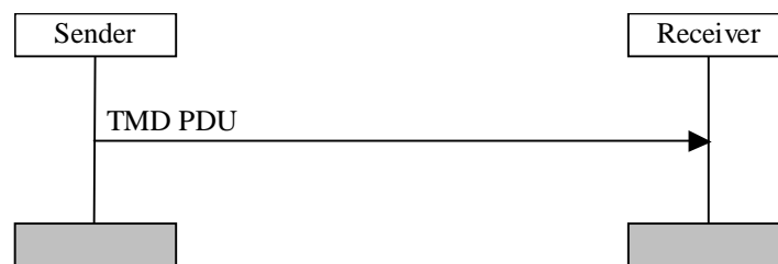
Figure 11.1: Transparent mode data transfer procedure
