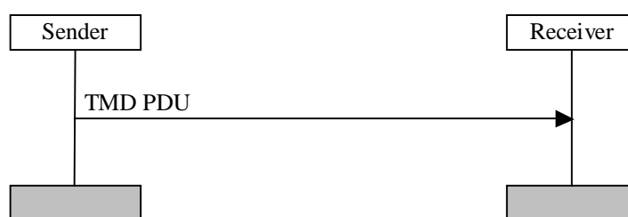
Figure 11.1: Transparent mode data transfer procedure
