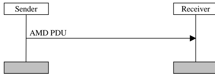
Figure 11.3: Acknowledged mode data transfer procedure
