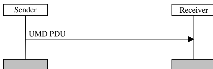
Figure 11.2: Unacknowledged mode data transfer procedure
