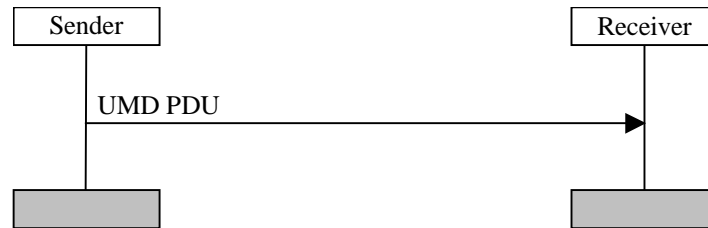
Figure 11.2: Unacknowledged mode data transfer procedure
