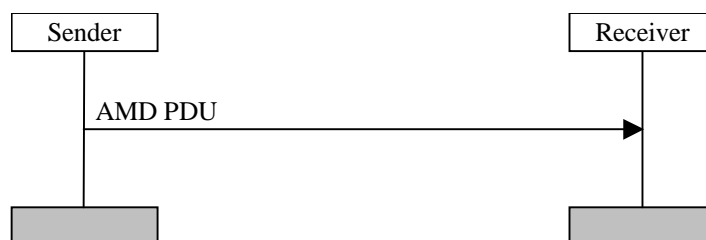
Figure 11.3: Acknowledged mode data transfer procedure
