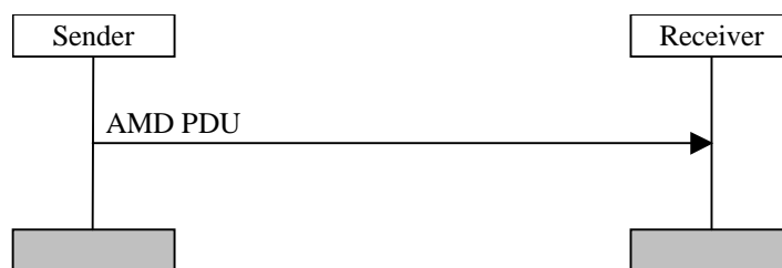
Figure 11.3: Acknowledged mode data transfer procedure
