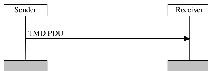
Figure 11.1: Transparent mode data transfer procedure
