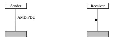
Figure 11.3: Acknowledged mode data transfer procedure
