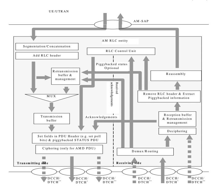
Figure 4.4: Model of an acknowledged mode entity
