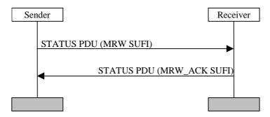
Figure 11.6: SDU discard with explicit signalling
