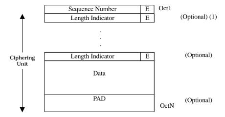
Figure 9.19: Ciphering unit for a UMD PDU
