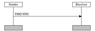
Figure 11.1: Transparent mode data transfer procedure
