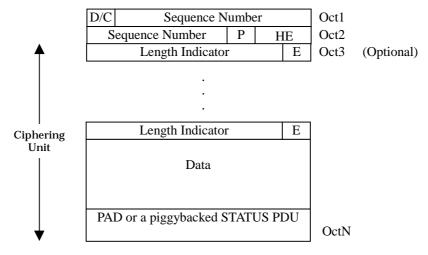
Figure 9.20: Ciphering unit for an AMD PDU
