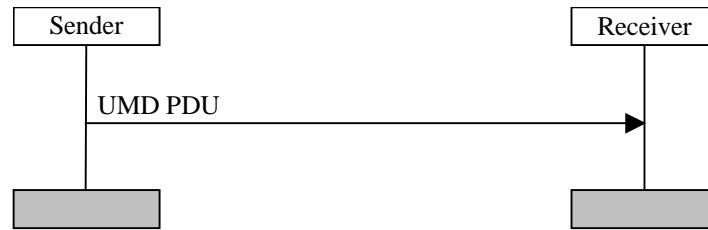
Figure 11.2: Unacknowledged mode data transfer procedure
