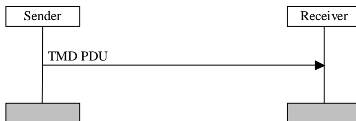
Figure 11.1: Transparent mode data transfer procedure
