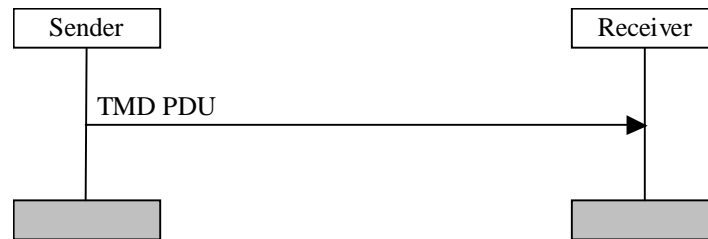
Figure 11.1: Transparent mode data transfer procedure
