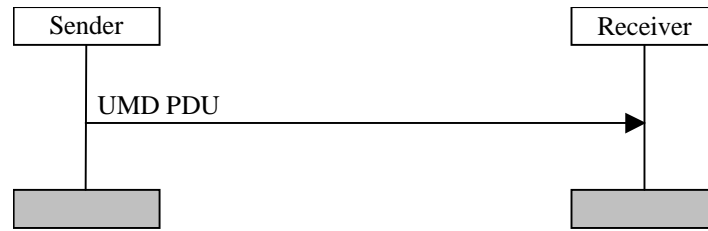
Figure 11.2: Unacknowledged mode data transfer procedure
